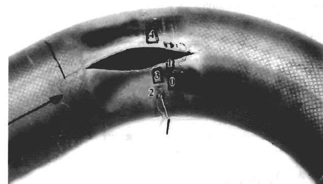
Fig. 6—Photograph of burst WN tube after failure illustrating strain gage locations.
